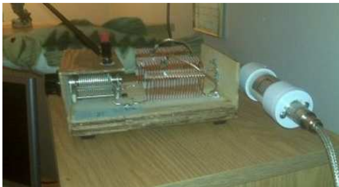
Fig. 1 Parallel LC Tuner with input 1:1 Choke **Note: Coils built via KOFF article on eHam.net
