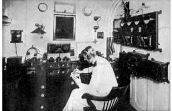
Radio room with spark gap transmitter on board the RMS Titanic, launched 31 May, 1911
